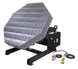
rotate the worktable with variable speed in both directions and change the angle of the main frame. Control is achieved through a foot pedal. The self-locking drive ensures that the rotating disc halts in any position. The positioner's mechanisms enable rotation around its own axis and deviation of the rotator up to 140° from the horizontal, while the tilt angle after mounting the tabletop is 90°. Control interface: manual panel + foot pedal (on separate cables).
