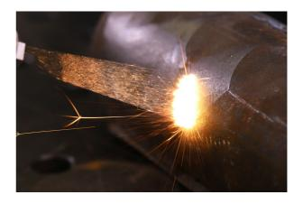
Copper and aluminum are materials with a high reflectivity coefficient and should not be subjected to the laser cutting process.
