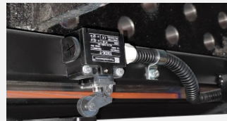
limit switch - crushing protection
