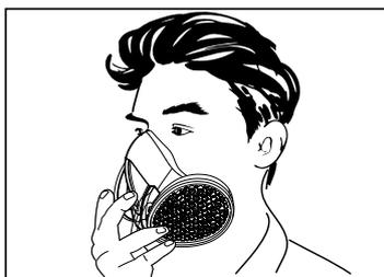
**A2** Loosen the head harness. Hold the half mask in the position over nose and mouth.
