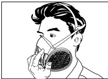
**A5** Press the palm of your hand over the exhalation valve cover and exhale gently. If no air leaks are being noticed between face and mask a proper fit has been achieved. If a leak has been detected reposition the respirator and readjust the tension of the head harness to eliminate leakage. Repeat the fit check.
