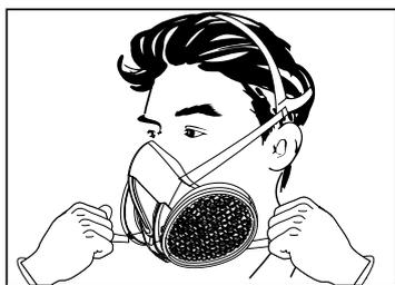
**A4** Release the inferior head harness and place it on neck, then pull the head harness to proper position to get a good seal.
