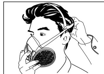
**A3** Place the superior head harness on the top of the skull. If necessary, readjust the head harness.
