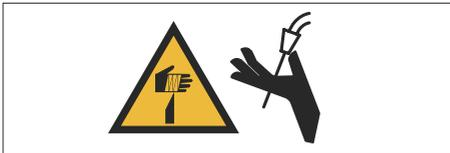
Accidental pressing of the button on the welding torch can cause welding wire to advance in an uncontrolled manner. The welding wire tip may be sharp.
