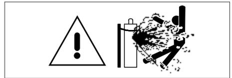
In case compressed gases are used in the work place, apply special safety measures to prevent dangerous situations.
