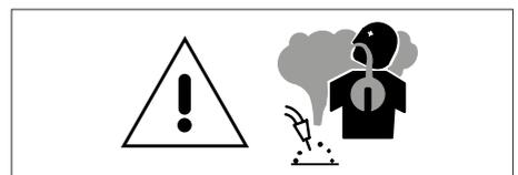
Arc welding and allied processes produce welding fume which may pollute the atmosphere surrounding the work. Welding fume is a varying mixture of airborne gases and fine particles which, if inhaled or swallowed, constitute a health hazard.
