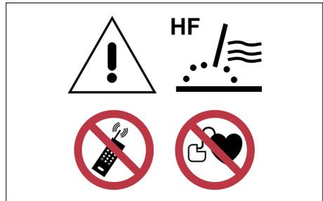
As welding by the TIG method or plasma cutting involves high frequency ignition, it can interfere with mobile phones, radio equipment, TV equipment or improperly protected computers and industrial robots, which leads to total disabling of such devices.
