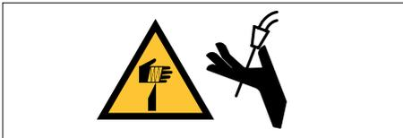
Accidental pressing of the button on the welding torch can cause welding wire to advance in an uncontrolled manner. The welding wire tip may be sharp.
