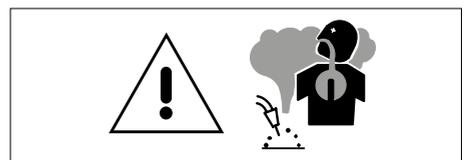
Arc welding and allied processes produce welding fume which may pollute the atmosphere surrounding the work. Welding fume is a varying mixture of airborne gases and fine particles which, if inhaled or swallowed, constitute a health hazard.
