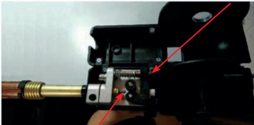
11. Pull the trigger to drive the wire down the neck until it exits the contact tip.
