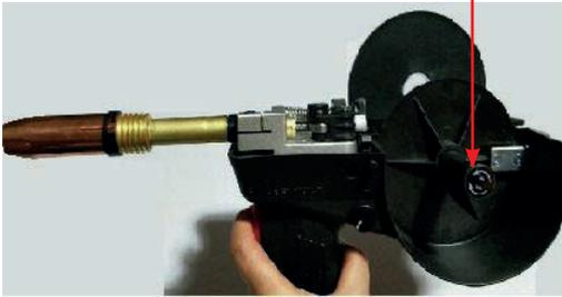
10. Feed the wire through the drive rolls and into the inlet guide tube. Tighten the wire tension swing arm.
