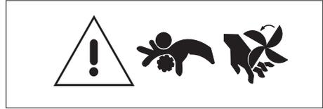
All protective elements and device housing should be in place and in good technical condition. Keep your hands, hair, clothes and tools away from gear wheels, fans and other moving parts during their operation.
