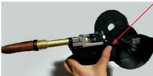
9. Place a spool of wire inside the spool holder on post.
