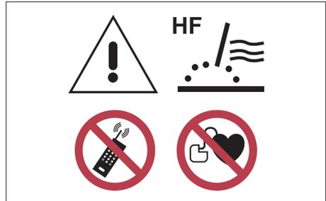
As welding by the TIG method or plasma cutting involves high frequency ignition, it can interfere with mobile phones, radio equipment, TV equipment or improperly protected computers and industrial robots, which leads to total disabling of such devices.
